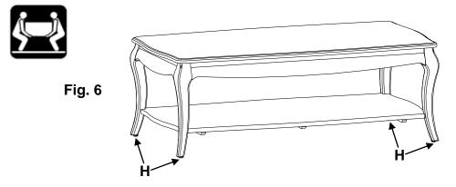
7. Place the table at its final destination. To level the table, rotate the Adjustable Glides (H) found on the bottoms of the legs. See Figure 6.
