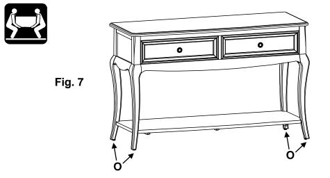
8. Place the table at its final destination. To level the table, rotate the Adjustable Glides (O) found on the bottoms of the leg assemblies. See Figure 7.
