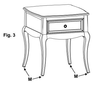
4. Place the table at its final destination. To level the table, rotate the Adjustable Glide (M) found at the bottom of each leg assembly. See Figure 3.
