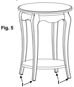
6. Place the table at its final destination. To level the table, rotate the Adjustable Glides (I) found on the bottoms of the legs. See Figure 5.
