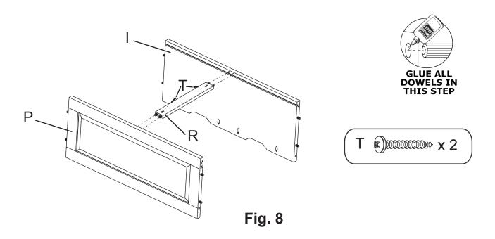
8. Spread a thin film of glue in the dowel holes in the Small Front Panel (P) and Small Lower Back (I). Insert Bottom Support (R) and gently tap with a padded hammer. Using the pocket holes as guides, attach with two #8x11/4" Pan Head Screws (T). See Figure 8.
