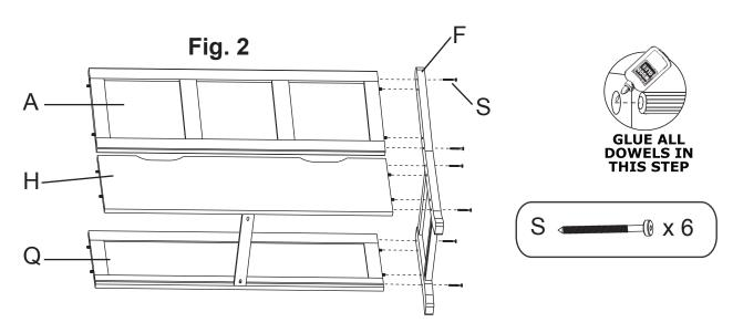
2. Spread a thin layer of glue in the dowel holes in one of the the Left Side Assemblies (F). Insert the Large Upper Back (A), Large Lower Back (H) and Large Front Panel (Q) and gently tap with a padded hammer. Quickly wipe away any excess glue with a damp rag. Using the provided Hex Wrench (Z), attach with six ½"x63mm Hex Screws (S). See Figure 2.
