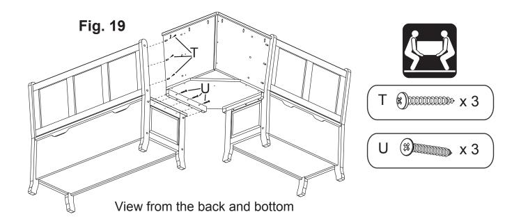
19. Turn the short bench and corner seat assembly right-side up and insert the dowels on the corner seat assembly into the long bench. These dowels do not need to be glued. Using the pre-drilled holes as guides, secure corner back seat/short bench assembly to the long bench with three #8x1½" Pan Head Screws (T) and three #8x1½" Black Screws (U) as shown in Figure 19.
