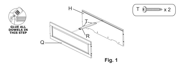
1. Spread a thin film of glue in the dowel holes in the Large Front Panel (Q) and Large Lower Back (H). Insert Bottom Support (R) and gently tap with a padded hammer. Using the pocket drilled holes as guides, attach with two #8x11/4" Pan Head Screws (T). See Figure 1.
