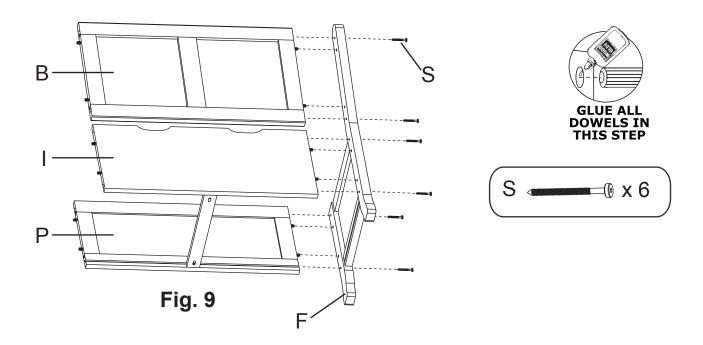
9. Spread a thin layer of glue in the dowel holes in the remaining Left Side Assembly (F). Insert the Small Lower Back (I), Small Front Panel (P) and Small Upper Back (B) and gently tap with a padded hammer. Quickly wipe away any excess glue with a damp rag. Using the provided Hex Wrench (Z), attach with six 1/4"x63mm Hex Screws (S). See Figure 9.
