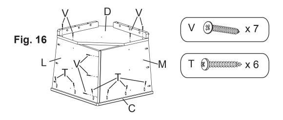
16. Using the pocket holes as guides, secure the Left Back Corner (L) and Right Back Corner (M) to the Corner Top (C) with six #8x1¼" Pan Head Screws (T). Using the pre-drilled holes as guides, secure the Left Back Corner (L) to the Right Back Corner (M) with three #8x1¼" Black Screws (V). Secure the Corner Seat (D) to the Left/Right Back Corners with four #8x1¼" Black Screws (V). See Figure 16.
