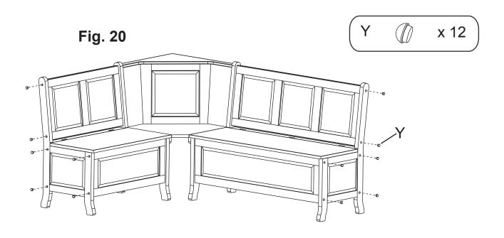
**19.** Glue Wood Buttons (Y) into the exposed holes. See Figure 20.
