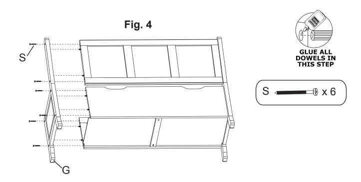
**4.** Spread a thin layer of glue in the dowel holes in one of the Right Side Assemblies (G) and attach to the bench assembly. Gently tap with a padded hammer and quickly wipe away excess glue with a damp rag. Using the provided Hex Wrench (Z), insert six ½"x63mm Hex Screws (S). See Figure 4.
