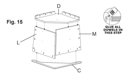
**15.** Spread a thin layer of glue into the two dowel holes in the Corner Top (C) and insert the pre-attached dowel in the Left Back Corner (L) and the one pre-attached dowel in the Right Back Corner (M). See Figure 15. Spread a thin layer of glue into the four dowel holes in the Corner Seat (D) and lower the Corner Seat (D) on to the two pre-attached dowels on the Left Back Corner (L) and Right Back Corner (M). Quickly wipe away any excess glue. See Figure 15.
