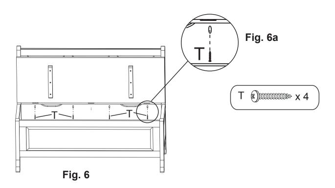
**6.** Open the Seat. Using the pocket holes as guides, attach Large Seat Assembly to Large Lower Back with four #8x1½" Pan Head Screws (T). See Figures 6 and 6a.
