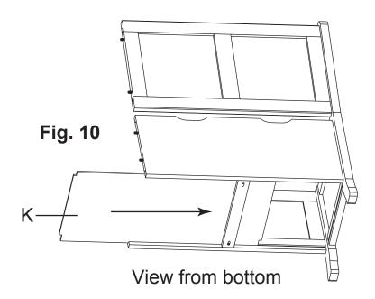
**10.** Slide Small Bottom (K) into grooves in Small Lower Back and Small Front Panel (I and P). See Figure 10.
