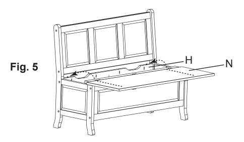
**5.** Spread a thin layer of glue in the two dowel holes on the bottom of the Large Seat Assembly (N). Place the Seat Assembly over the dowels on the Large Lower Back (H) and quickly wipe away excess glue with a damp rag. See Figure 5.
