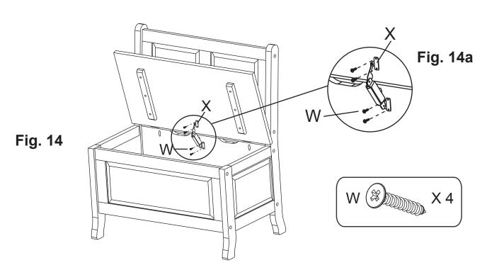
**14. The long arm of the Lid Support (X) must be attached to the Seat.** Position the Lid Support (X) over the pre-drilled holes in the Small Lower Back and Small Seat Assembly. Attach using four #5x5/8" Flat Head Screws (W). See Figures 14 and 14a.
