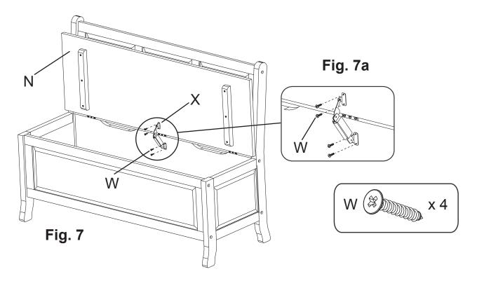
7. The long arm of the Lid Support (X) must be attached to the Seat. Position the Lid Support (X) over the pre-drilled holes in the Large Lower Back (N) and Large Seat Assembly. Attach using four #5x5/8" Flat Head Screws (W). See Figures 7 and 7a.
