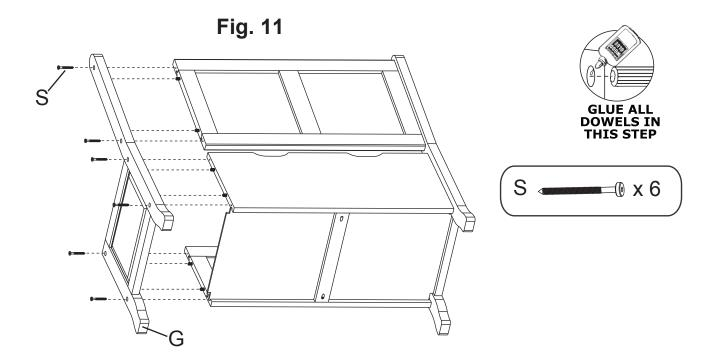
**11.** Spread a thin layer of glue in the dowel holes in the remaining Right Side Assembly (G) and attach to the bench assembly. Gently tap with a padded hammer and quickly wipe away any excess glue with a damp rag. Using the provided Hex Wrench (Z), insert six ½"x63mm Hex Screws (S). See Figure 11.
