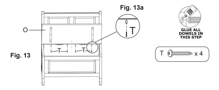
**13.** Open the Seat. Using the pocket holes as guides, attach Small Seat Assembly to Small Lower Back with four #8x1½" Pan Head Screws (T). See Figures 13 and 13a.
