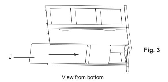
**3.** Slide Large Bottom (J) into grooves in Large Lower Back and Large Front Panel (H and Q). See Figure 3.
