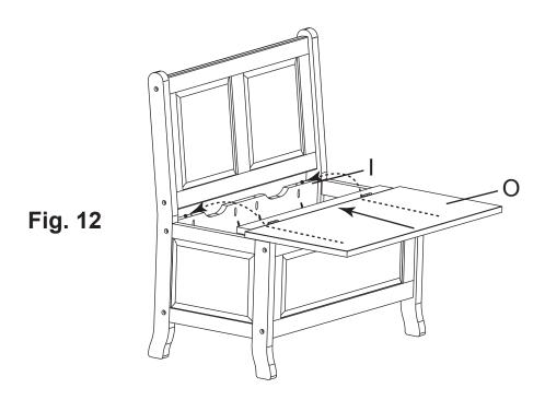
**12.** Spread a thin layer of glue in the two dowel holes on the bottom of the Small Seat Assembly (O). Place the Seat Assembly over the dowels on the Small Lower Back (I) and quickly wipe away excess glue with a damp rag. See Figure 12.
