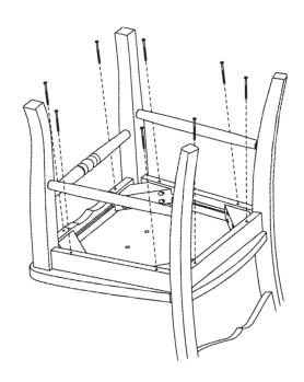
Lay the Seat face down on a clean protected surface, with the back of the seat hanging over the edge.
