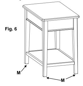
7. Place the table at its final destination. To level the table, rotate the Adjustable Glides (M) found on the bottoms of the legs. See Figure 6.
