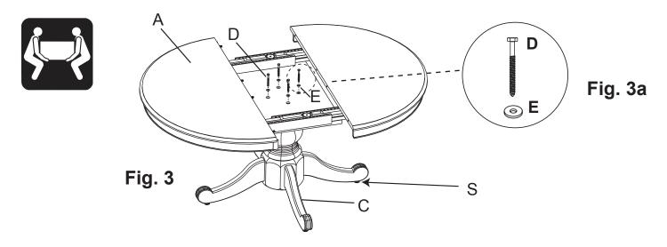
Turn the Pedestal right-side up and line up the pre-drilled holes in the Top Assembly to the pre-drilled holes in the pedestal. Attach using four 5/16"x3" Lag Bolts (D) and four 5/16" Washers (E) as shown in Figures 3 and 3a. To level the table, turn the Adjustable Glides (S) on the bottom of each Foot (C).
