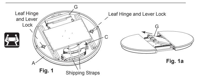
Place the Top Assembly (A) upside down on a clean protected surface and remove the Feet (C) as seen in Figure 1 and place them off to the side. Unlatch the locks. Turn the top assembly right-side up and pull open the table ends to expose the Leaf Assembly (G). Remove the Leaf Assembly (G) and set it off to the side. See Figure 1a. Remove the foam now, but when you store the leaf, place the foam in between the folded leaves. This will help protect its surface.
