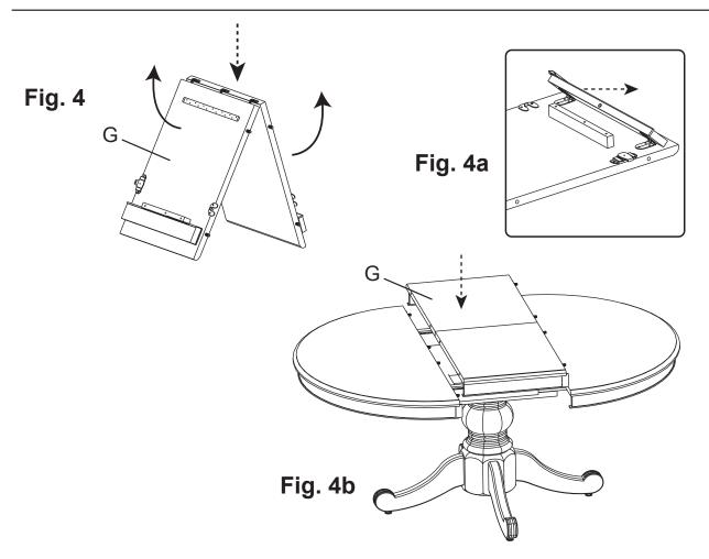
4. To insert the leaf, flatten out the Leaf Assembly (G) as shown in Figure 4. Flip open the Apron on each end of the leaf assembly as in Figure 4a and turn it right-side up. Place it in the open space between the table ends and line up the guide pins and holes. Gently push the table ends until the leaf fits snugly. See Figure 4b. Close the locks that are underneath the table.
