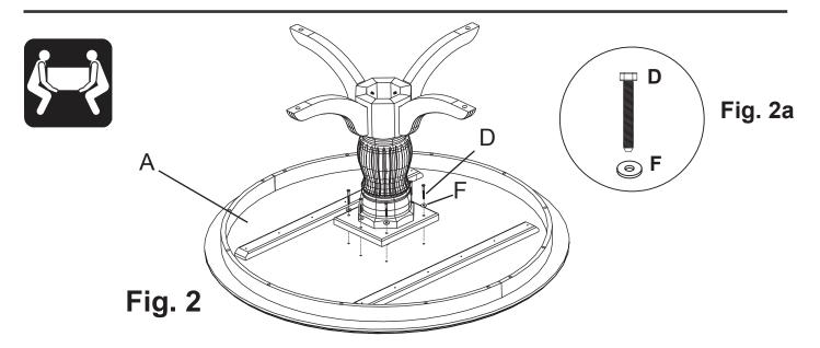
2. Turn the Top Assembly (A) upside down on a clean, protected surface. Align the holes in the Pedestal Assembly (B) to the holes in the Top Assembly (A) as in Fig. 2 and attach with ½" Flat Washers (F) and ½" x 1¾" Hex Bolts (D). See Fig. 2a. Turn upright and adjust levelers on the feet if needed.
