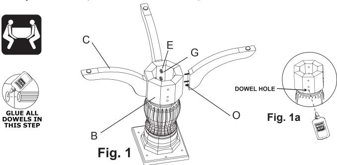
1. Turn the Pedestal Assembly (B) upside-down so that the Top Support is on the floor. Apply a light film of glue into each of the four dowel holes in the Pedestal Asssembly (see Fig. 1a). With a damp rag, quickly wipe off any excess glue. Insert the Foot (C) into the holes on the Pedestal Assembly (B). The Hanger Bolts should go all the way through the base. Gently tap feet into place with padded hammer. Fasten in place with 5/16" washer (E) and 3/8" Hex Nut (G).
