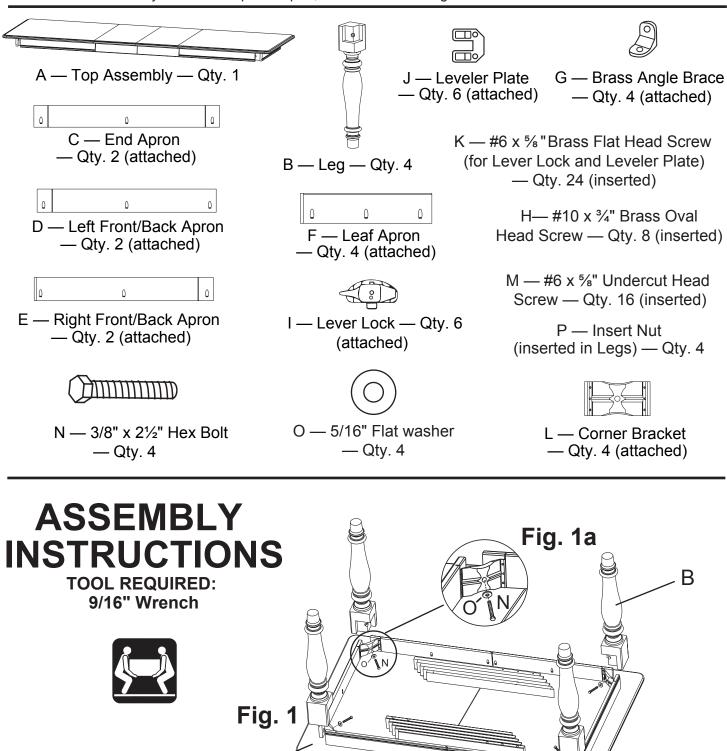
Place Top Assembly (A) upside-down on a clean, protected surface. Position Legs (B) on Top Assembly (A) outside of and against the corners of the aprons. Insert 3/8" x 2<sup>1</sup>/<sub>2</sub>" Hex Bolt (N) through Washer (O) and Bracket, and screw into Leg (B). Tighten bolts. See Figure 1a. Turn your table upright.
