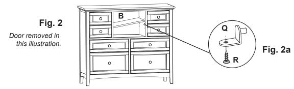
2. Install the Adjustable Shelf (B) at the desired location using the Shelf Brackets (Q). See Figure 2. Attach the shelf to the shelf brackets by inserting #6 x 1/2" Undercut Screw (R) through the bottom of the shelf bracket and into the shelf. See Figure 2a.
