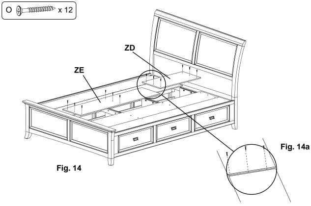
Place three #8x1-1/4" Black Screws (O) along the seam between the Deckboards (ZD) and (ZE). See Figure 14a.
