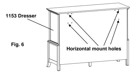
Using the predrilled holes on the back of the Dresser as guides, attach the two Mirror Supports (E) with four M4 x 41 Machine Screws (K). The upper screws will be inserted into the 3<sup>rd</sup> hole from the top and the lower screws will be inserted into the 1<sup>st</sup> hole from the bottom of the Mirror Supports. See Figures 7 and 7a.
