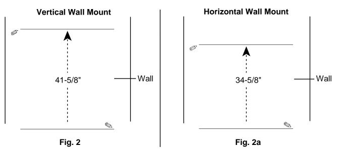
Locate two studs in the wall behind the space where you want to hang your Mirror. Affix the Mirror Wall Bracket (G) into the studs with two #8 x 1-3/4" Pan Head Screws (H). If you cannot locate two studs, purchase the proper wall attachment hardware for your type of wall and secure the bracket. See Figure 3.
