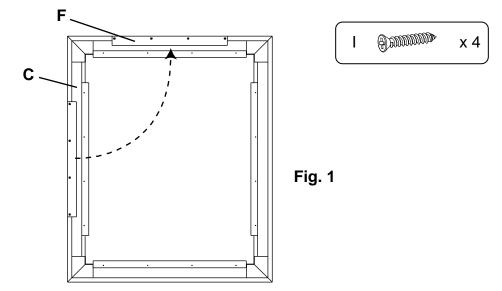
2. Determine where you want the bottom of your mirror to end and draw a faint pencil line on the wall. For a vertical placement, use a tape measure and measure up 41-5/8" from that mark. Draw a faint line. For a horizontal placement, measure up 34-5/8". Draw a faint line. The top line is where you attach the Mirror Wall Bracket (G). If you like, you can erase the faint bottom pencil mark. See Figures 2 and 2a.
