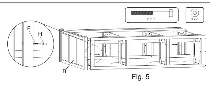
Assemble the Footboard (B) to the Pedestal Assembly as shown in Fig. 5. using 1/4" x 3" Hex Bolt (F) and Washer (H). 6. Repeat step 5 to assemble the Headboard (A) to the Pedestal Assembly as shown in Fig. 6.
