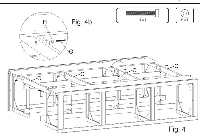
Place 4 Trestles (C) in between Pedestals and insert 1-1/4" Hex Bolt (G) and washer (H) as shown in Fig. 4b. Finger tighten only.
