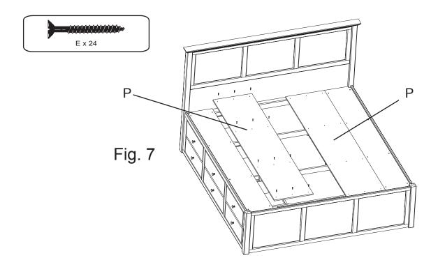
8. Place Deckboards (P) as shown in Fig. 7 and secure with #8 x 1" Screw (E).
