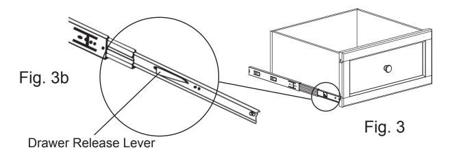
3. Remove Drawers (J & K) from Pedestal Kits (I). To remove drawers, push up on the left side of the Drawer Release Lever while pushing down on the right Drawer Release Lever (see Fig. 3b). Note where each drawer came from to ensure correct re-installation. (Positions are marked on drawer backs.)
