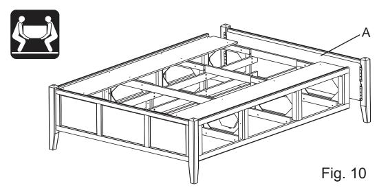
10. Attach Headboard (A) to Pedestal Assembly as in previous step. *NOTE: NOW TIGHTEN ALL BOLTS ON TRESTLES.*
