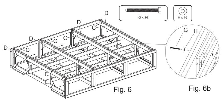
6. Place the remaining Trestles (C and D) on the Pedestal Assembly. Face the Trestles with T-Nuts (D) toward the ends of the Assembly from the center as shown in Fig 6. Insert 21/2" Hex Bolt (G) and Washer (H). See Fig. 6b. DO NOT TIGHTEN BOLTS **UNTIL FINAL ASSEMBLY IN STEP 10.**
