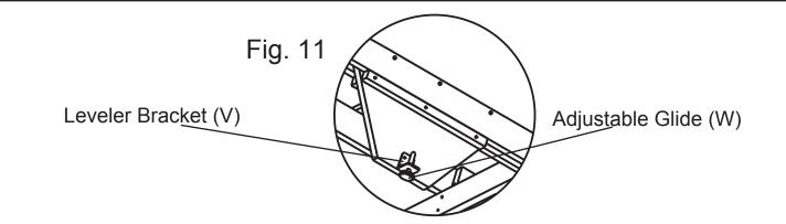
11. Adjust Glides (W) on the Foot Assemblies (U) so the Glides just touch the floor.
