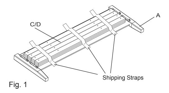
1. Remove the Trestles (C/D) from the back of the Headboard (A) as seen in Fig. 1 and place them off to the side.
