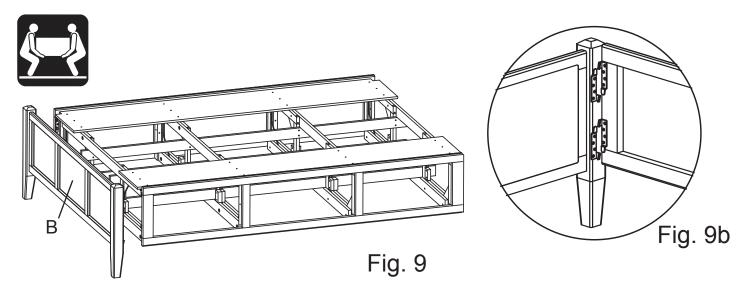
9. Attach the Footboard (B) to the Pedestal Assembly as in Fig. 9. Align brackets as shown in Fig. 9b, and slide the Pedestal Assembly down on to the Footboard (B).
