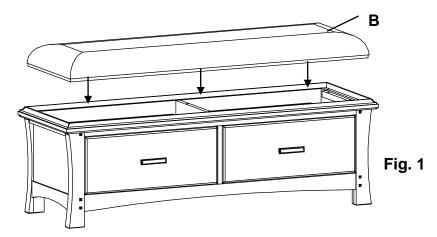
2. To attach your seat, remove the drawers, noting where each drawer came from to ensure correct reinstallation. To remove the drawers, push up on the left Drawer Release Lever while pushing down on the right Drawer Release Lever (see Figures 2a and 2b). Place the unit upside down. Using the predrilled holes as guides, attach the Seat (B) with the six #8 X 1-1/4" Pan Head screws (H) as shown in Figures 2 and 2c. Turn the unit upright and install the drawers.
