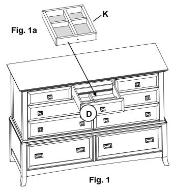
2. There is a secret storage area in the Center Drawer (D). To access this storage, open the upper right Middle Drawer (E). Reach in until you find the Hinged Drawer Stop (Va) that is attached to the bottom of the Center Drawer (D). Pull the Hinged Drawer Stop (Va) forward and then pull the center drawer (D) out far enough so you can access the concealed storage space. To close the drawer, just push it shut. See Figure 2.
