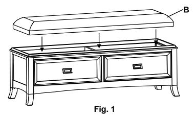
2. To attach your seat, remove the drawers, noting where each drawer came from to ensure correct reinstallation. To remove the drawers, push up on the left Drawer Release Lever while pushing down on the right Drawer Release Lever (see Figures 2a and 2b). Place the unit upside down. Using the predrilled holes as guides, attach the Seat (B) with the six #8 X 1-1/4" Pan Head screws (M) as shown in Figures 2 and 2C. Turn the unit upright and install the drawers.
