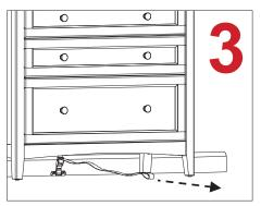
Push furniture against the wall and reach underneath to grasp the loop. Pull the loop end until tight.
