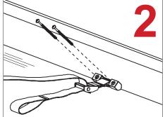
Loosen the strap and attach the bracket at a 45° angle under the baseboard in the desired location.
